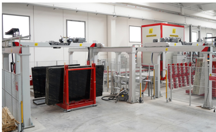
IT Butterfly B416 con carico/scarico su cavalletti singoli mobili o su supporti doppi girevoli . EN Butterfly B416 with loading/unloading on individual and mobile slab holder stands or on double rotating supports .
