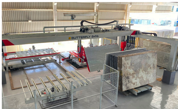
IT Butterfly B416 con carico/scarico su cavalletti singoli mobili o su supporti doppi girevoli . EN Butterfly B416 with loading/unloading on individual and mobile slab holder stands or on double rotating supports .
