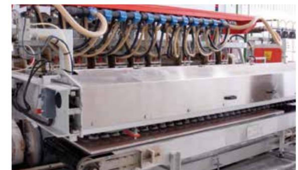
*After the cutting, the finished elements only are caught and deposited on the outlet conveyor belt by a suction cups system.*
