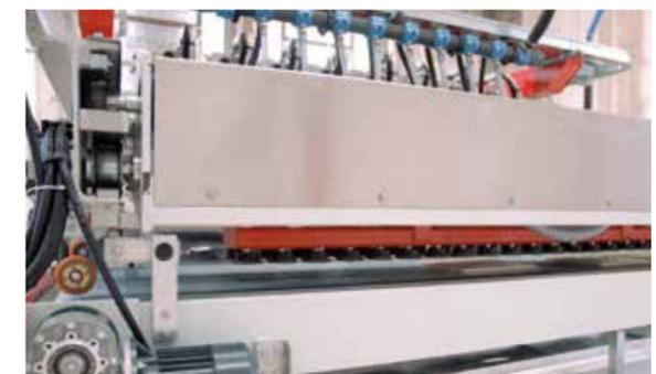
*A set of sensors mounted at the machine entry detects the strip head so the position of the first disc matches the first cut.*
