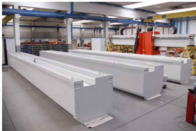
*The vertical discs group moves along a bridge built with a large honeycomb shaped structure which is free from bending and is machined with one sole positioning on the tool machine.*
