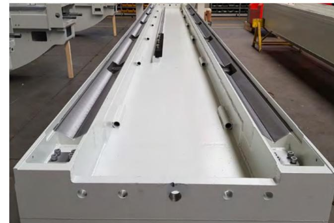
*The exclusive "V" shaped double guides which allow the sliding of the disc-holder trolley, constantly lubricated in oil bath, are machined onto the upper part of the bridge.*
