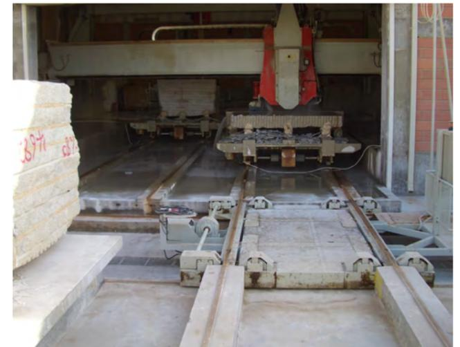
*The trolley is moved by a gear motor, fixed on the lower part, which allows the trolley to smoothly move on special railways perfectly positioned to have a linear sliding when the trolley is fully loaded.*
