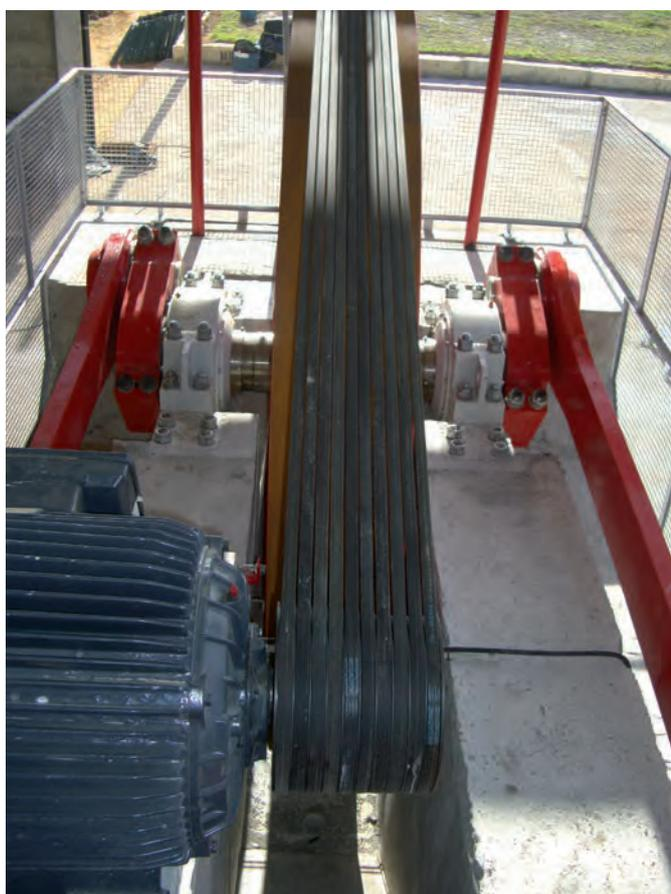
*The heavy eight-spokes flywheel that controls the alternate blades holder frame movement is fixed onto a battery composed of:*
