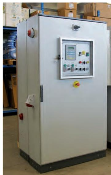
*The electric panel, air-conditioned by heat exchanger, is water and dust proof in compliance with IP 54 standards.*
