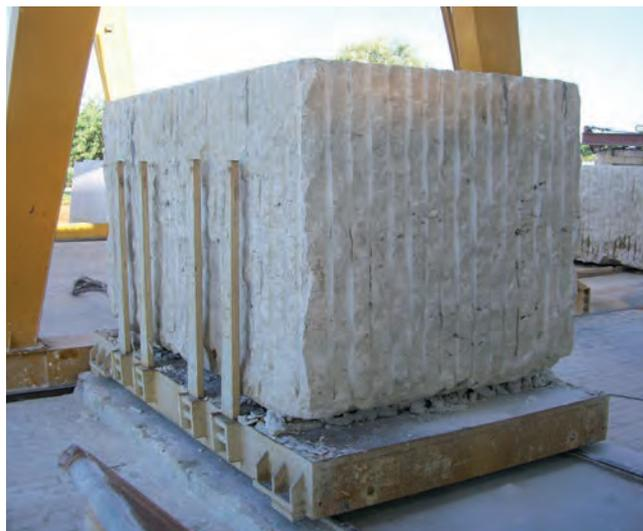
*The motorized block carrier trolley is equipped with hardened wheels and during the cutting phase it is automatically locked to the platform by a racks system.*
