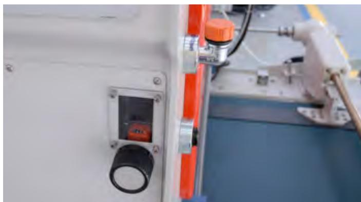
*The beam transversal stroke can be adjusted during the machine running as well, by acting on a mechanical manual indicator placed in the machine front position.*
