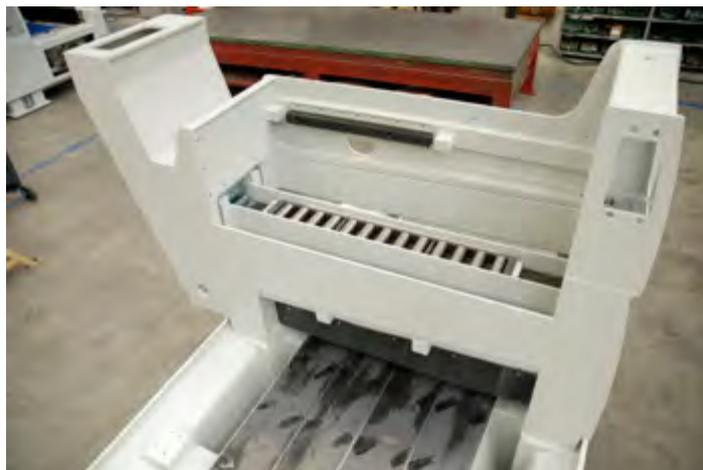
*Two side bridges house the oil bath hardened and ground rolls and allow the beam translation sliding.*
