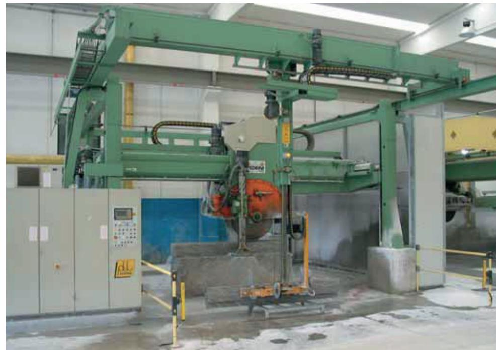
■ The cutting parameters are pre set through the key board. Work cycles are controlled through PLC, positions and parameters are visualized in real time on display.
