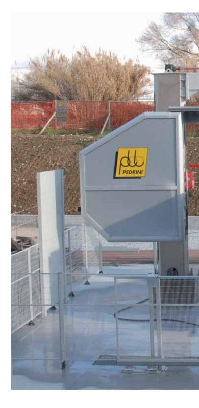
Pedrini SINGLEWIRE JUPITER GS210 performs single cuts on marble, granite and natural stones blocks up to 4200 mm long. It can be used both for squaring and for cutting blocks into slabs.
